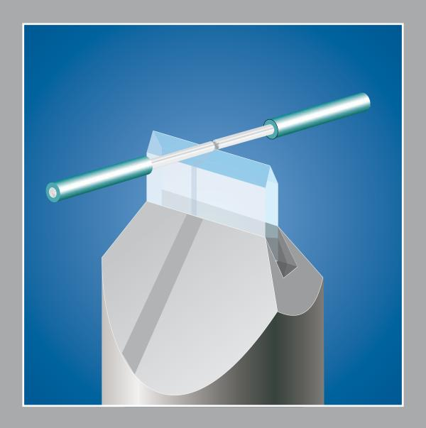
Diamond cleavers for fibre optic scoring
